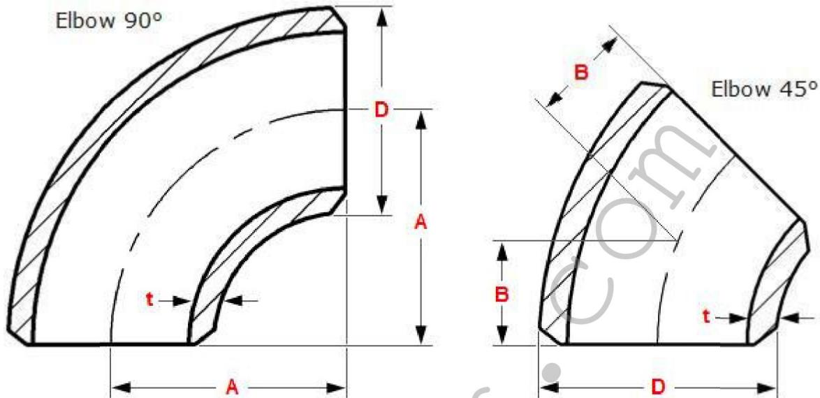
EEMUA 234 - Butt Welding Fittings connecting with EEMUA 234 Pipe
